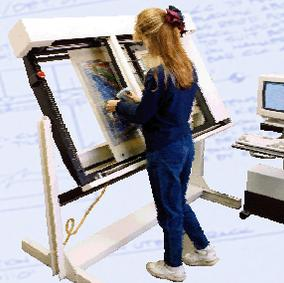
Semi-automatic wiring system for wiring of in-circuit fixtures.
