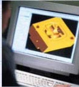
Fixture files are processed in CAD to assign test points, layout of UUT and any special machining. Data is then uploaded to the production equipment for manufacturing.
